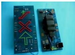
ESCALATOR DISPLAY BOARD
